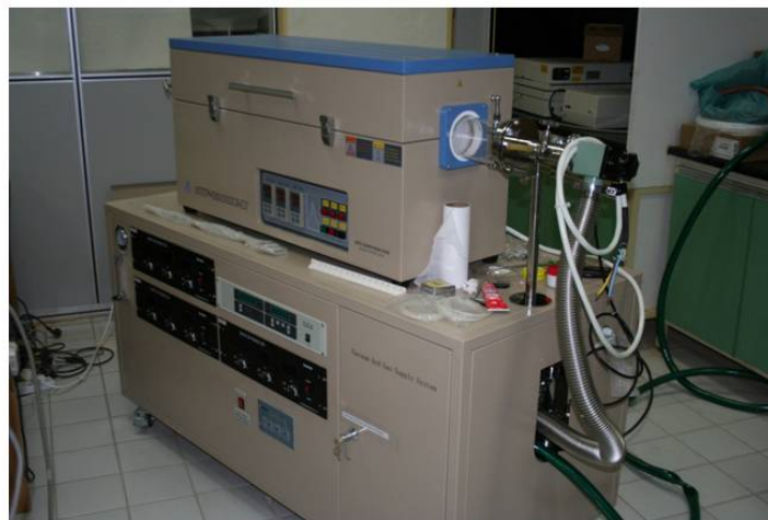
"Chemical Vapor Deposition (CVD) System for Carbon Nanotubes Synthesis (MTI Corporation, California, USA).
